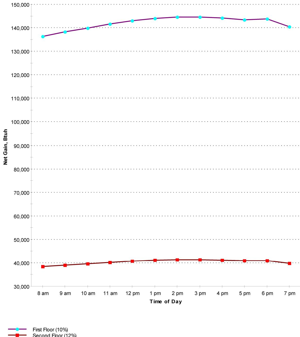
Note: Glass gain as a percent of net gain is shown in parenthesis. Although floor, roof, wall and door gains also vary throughout the day, for this graph and in Manual J glass gains are the only ones that fluctuate.
